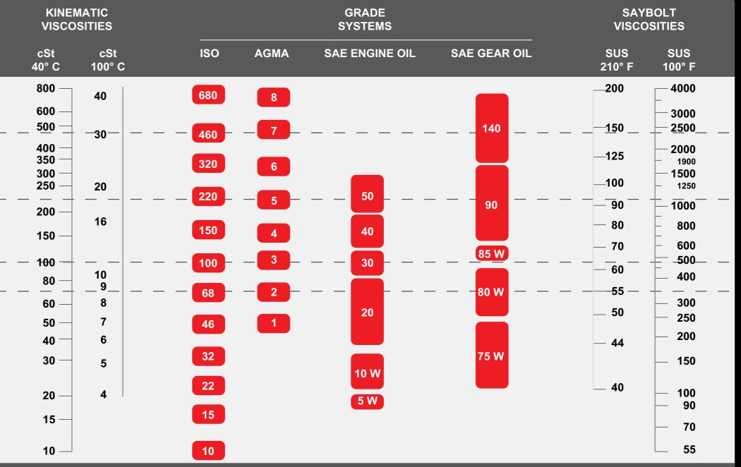
Viscosities can be related horizontally only. For example, the following oils have similar viscosities: ISO 460, AGMA 7 and SAE GEAR OIL 140. The viscosity/temperature relationships are based on 95 VI oils and are usable only for mono grade engine oils, gear oils and other 95 VI oils. Crankcase oils and gear oils are based on 100° C viscosity. The "W" grades are classified on low temperature properties. ISO oils and AGMA grades are based on 40° C viscosity.
